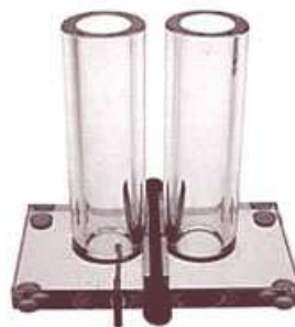
Typical gradient former casting chamber (165-2950)
